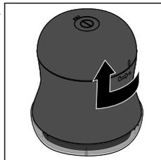
Twist the battery compartment lid clockwise and take it off.
