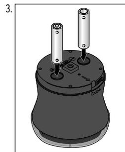
Insert the batteries as illustrated. Ensure that the polarity (+/-) is correct:
