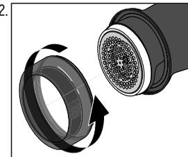
Twist the lint collector anti-clockwise to remove it.
