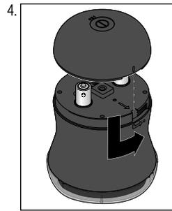
Place the battery compartment lid back on. The catch in the lid should fit into the slot marked with an arrow on the device. Then tighten the lid by turning it anti-clockwise.
